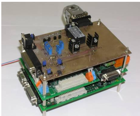
Fig. 7. DSP controller with resolver to digital add-on on the top
