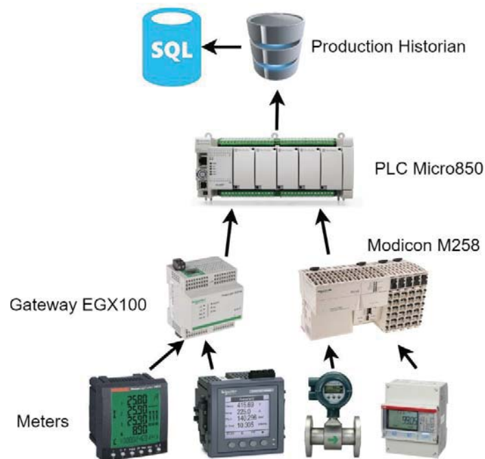
Figure 4: Proposed Data Flow Architecture
