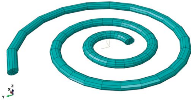
Fig. 1. Representative example of mechanical system - Fibonacci spring
