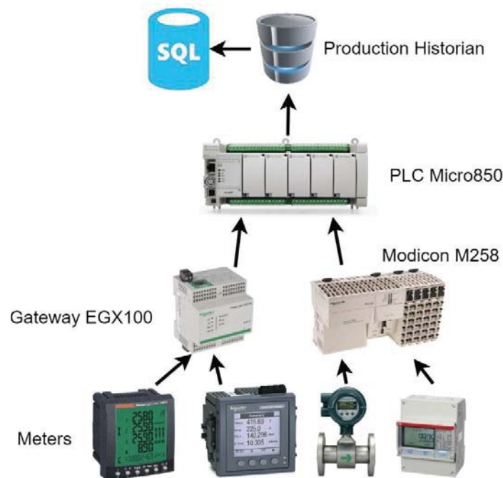
Figure 4: Proposed Data Flow Architecture
