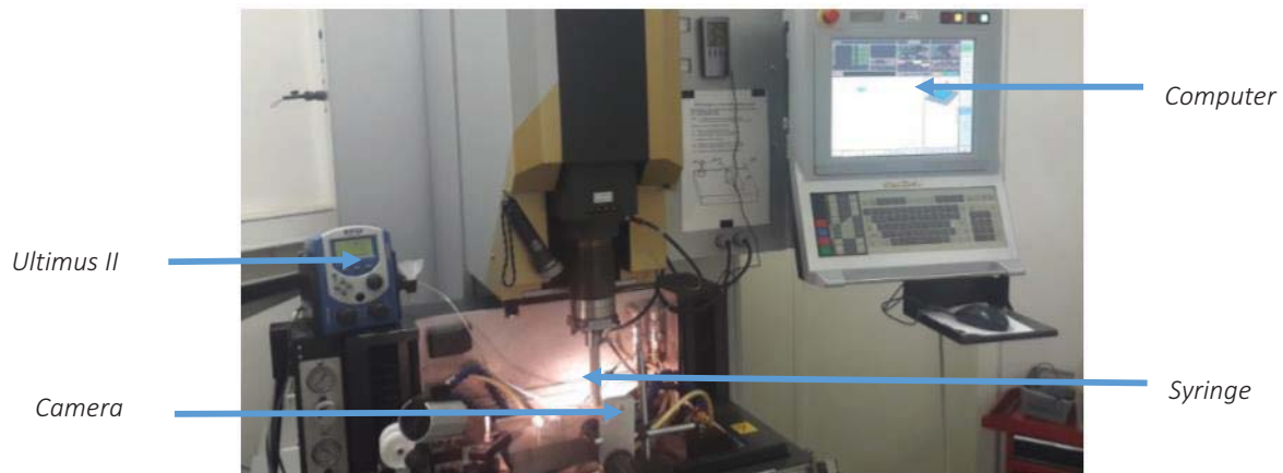
Fig.2. Experiment setup with the EDM
