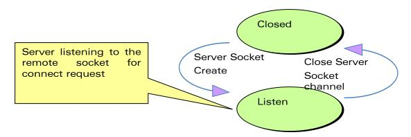
On reception of a connection request from a remote client socket, a server socket does the following,
