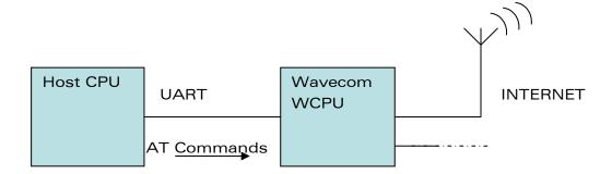
**Multiplexing:** Several sockets can be operating at once. The +WIPDATA command allows to temporarily identify the UART in data mode with a given socket. The data written on UART is transferred through the socket. The data which arrives on the socket can be read from the UART.
