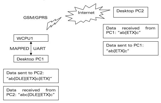
The above schematic explains how [ETX] characters which have a special meaning in WIP soft are handled on Wavecom Wireless CPU<sup>®</sup>.
