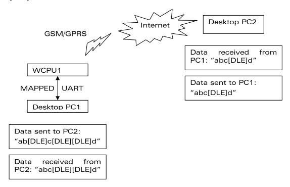
The above schematic explains how [DLE] characters which have a special meaning in WIP soft are handled on Wavecom Wireless CPU<sup>®</sup>.
